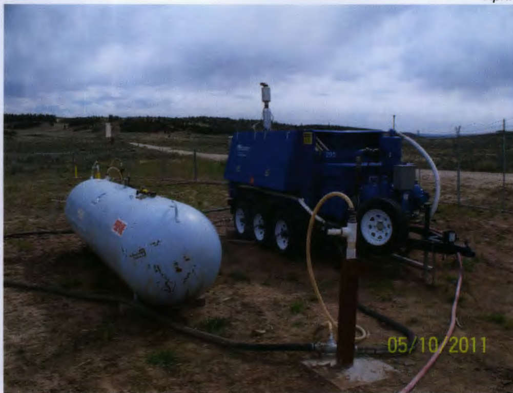
9. May 10, 2011: Facing SW, installed mobile ICE system and propane tank.
