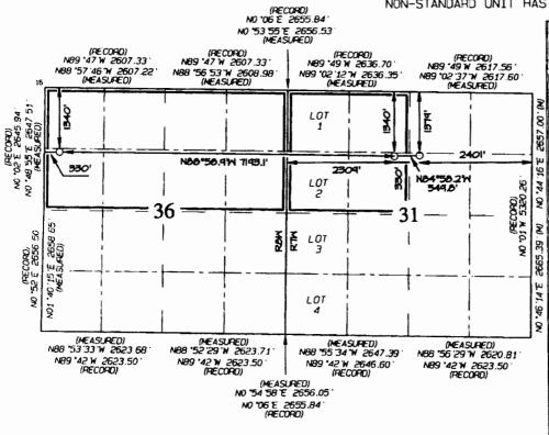
END-OF-LATERAL 1340 FML 330 FML SECTION 36, T23N, RBM LAT: 36, 18599 N LONG: 107, 64028 W DATUM NAD1927 LAT: 36, 18701 N LONG: 107, 64089 W DATUM: NAD1983 POINT-OF-ENTRY 1340 FNL 2309 FWL SECTION 31, T23N, R7W LAT: 36.18692 N LONG: 107.61591 W DATUM: NAD1927 LAT: 36.18684 N
