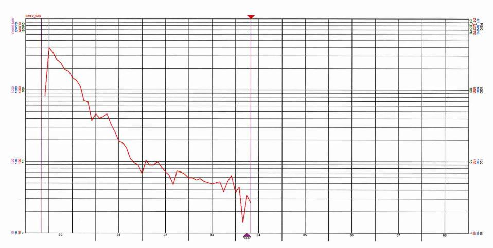
Ute Dome Morrison perfs from 2580'-2592' went off production due to pressure depletion. No production is expected from perfs from 2580'-2592' after plog drill out because they have been depleted.
