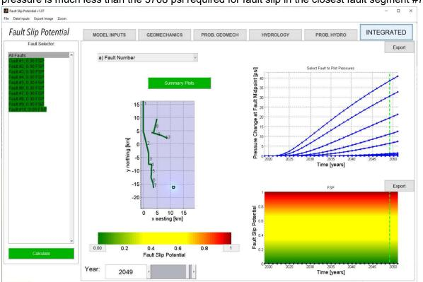
**Year 30 Fault Slip Probability** (0% for all fault segments after 30 years. 39 psi fault delta pressure is much less than the 3708 psi required for fault slip in the closest fault segment #7)
