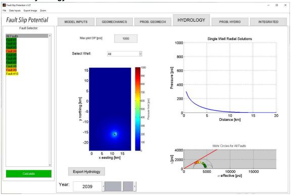
Year 20 Probabilistic Hydrology (note no crossover between blue delta-press. & green fault slip press.)
