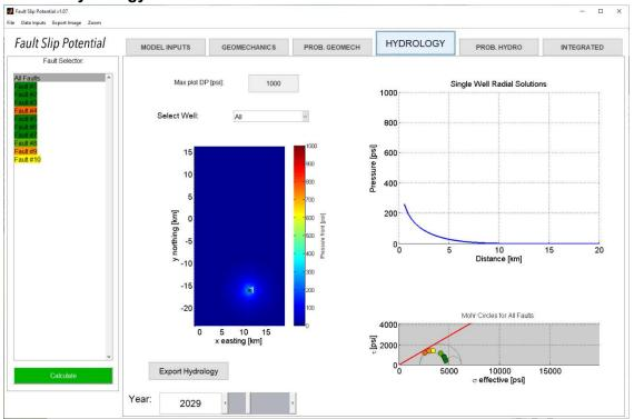
Year 10 Probabilistic Hydrology (note no crossover between blue delta-press. & green fault slip press.)
