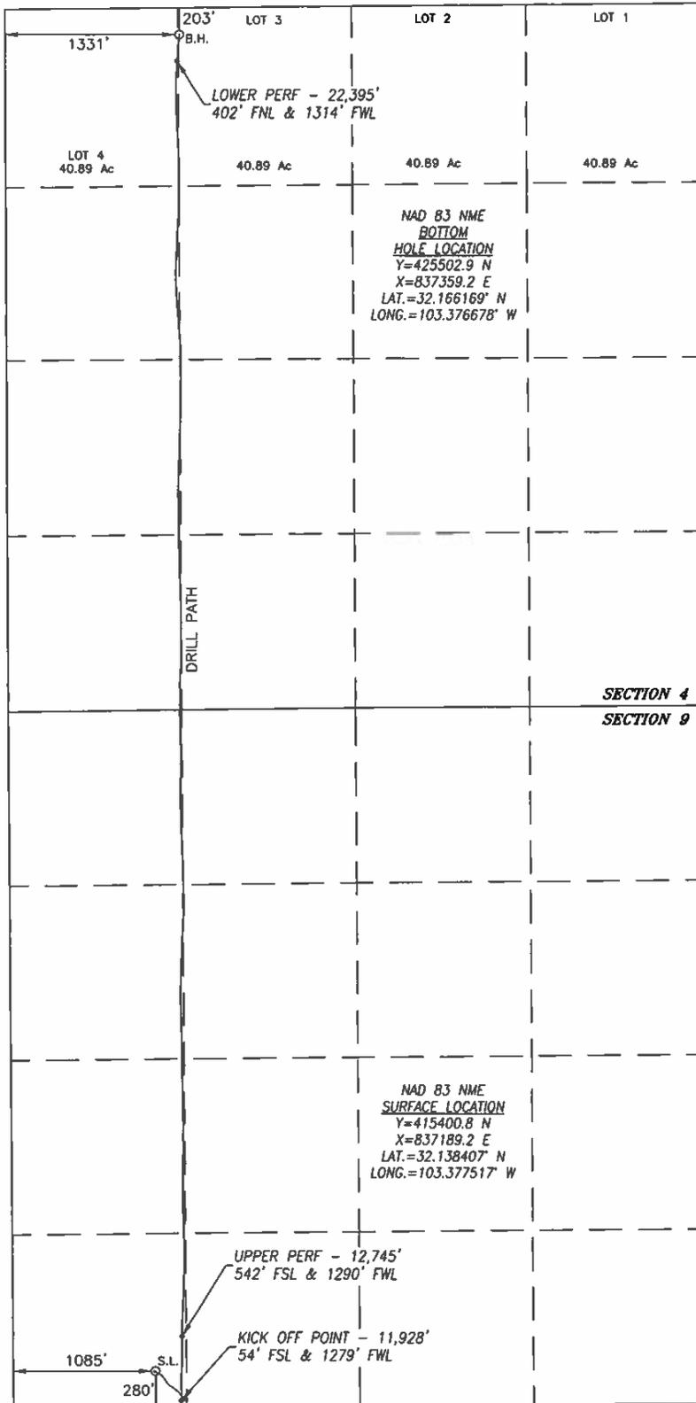
SURFACE INFO AND BOREPATH SHOWN HEREON IS BASED ON DIRECTIONAL SURVEY REPORT PROVIDED BY COG OPERATING, LLC FOR THE FEZ FEDERAL COM #703H SUPPLIED TO HARCROW SURVEYING, LLC ON NOVEMBER 14, 2019
