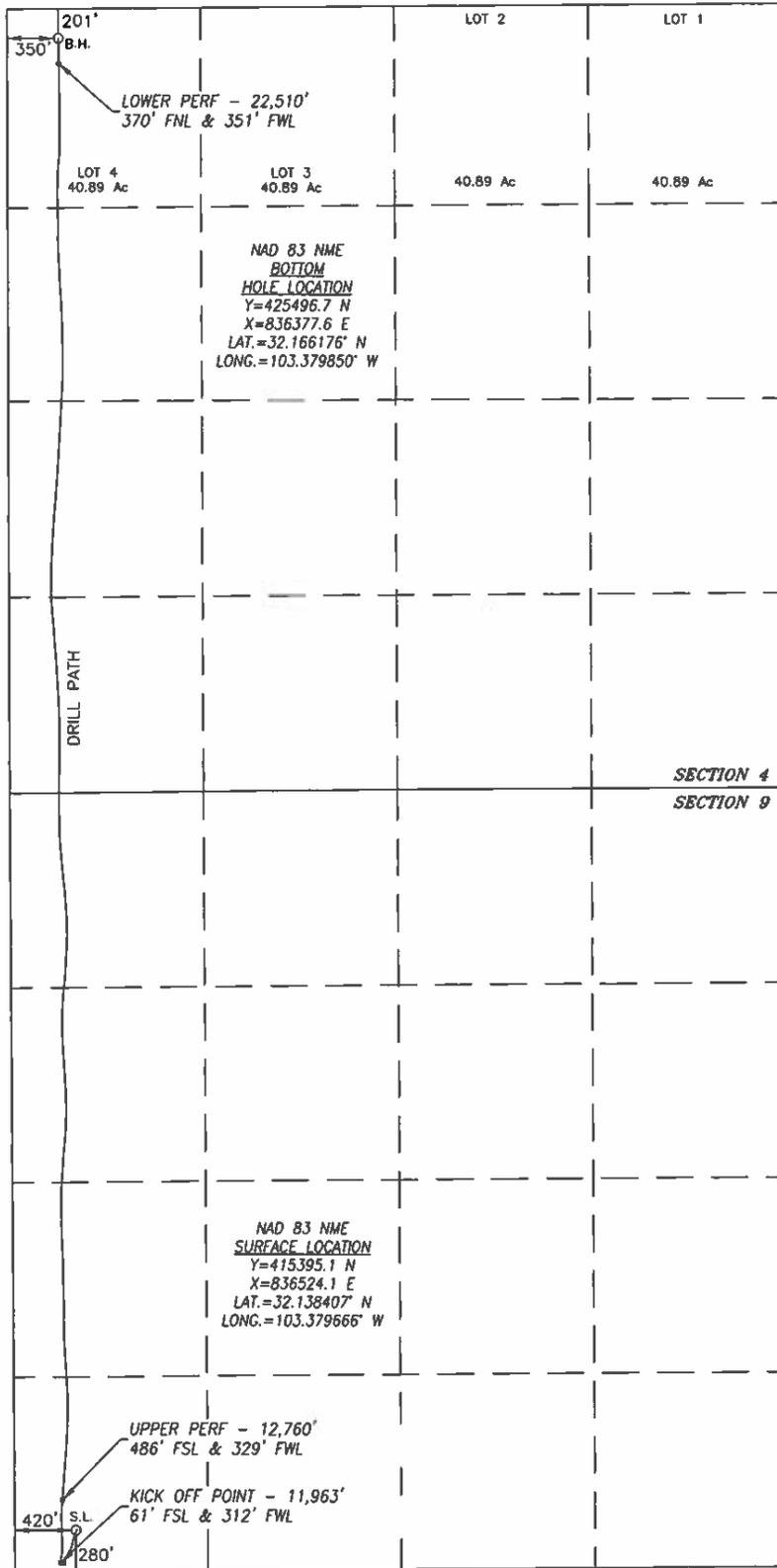
SURFACE INFO AND BOREPATH SHOWN HEREON IS BASED ON DIRECTIONAL SURVEY REPORT PROVIDED BY COG OPERATING, LLC FOR THE FEZ FEDERAL COM #705H SUPPLIED TO HARCROW SURVEYING, LLC ON NOVEMBER 16, 2019
