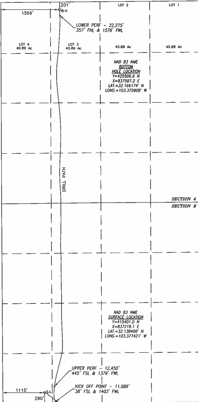
SURFACE INFO AND BOREPATH SHOWN HEREON IS BASED ON DIRECTIONAL SURVEY REPORT PROVIDED BY COG OPERATING, LLC FOR THE FEZ FEDERAL COM #702H SUPPLIED TO HARCROW SURVEYING, LLC ON NOVEMBER 18, 2019
