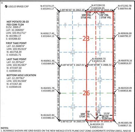
(2011), BASED FROM GPS OBSERVATIONS, OCCUPYING A WHS CONTROL POINT (5/8" REBAR), LOCATED AT NORTH: 456034.443, EAST: 653560.641, ELEVATION: 3101.4, DETERMINED BY AN OPUS SOLUTION ON MOVEMBER 9TH, 2019 2. DISTANCES DEPICTED HEREON ARE REPORTED AS GROUND DISTANCE IN US SURVEY FEET USING A COMBINED SCALE FACTOR OF 1.000220989 3. ELEVATIONS ARE OF NAVD 88 COMPUTED USING GEIOD 12B.
