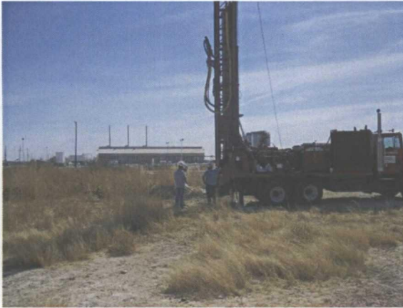
Drilling soil bores, facing east
