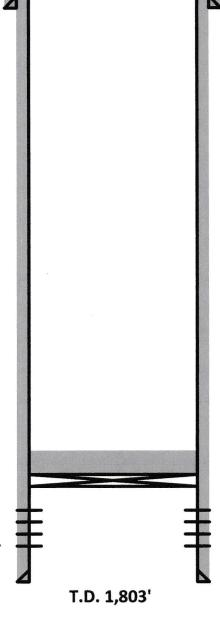
7 7/8" Hole. Set 5 ½" Csg. @ 1,803'. Cemented with 375 sx. Cement Circulated to Surface
