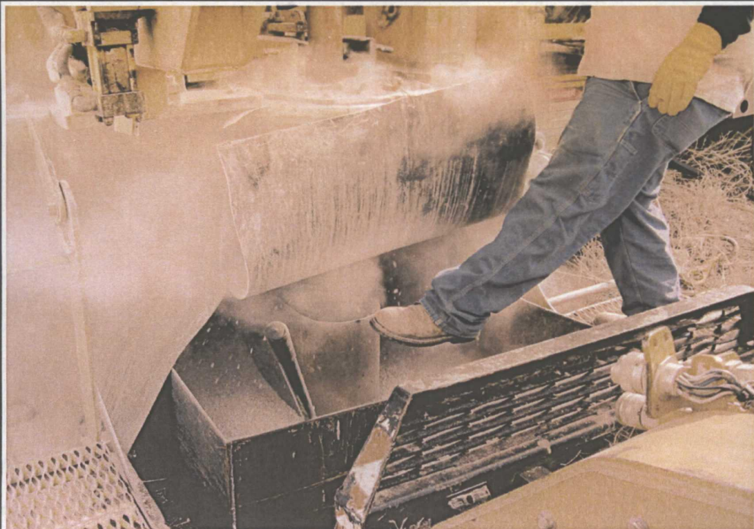
Air returns with cuttings while drilling
