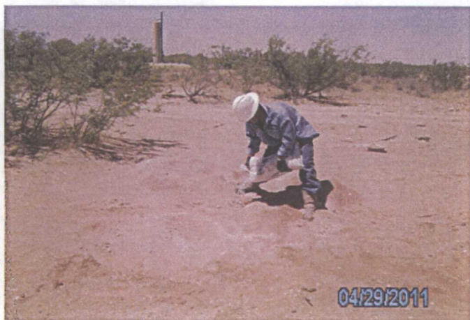
Plugging SB-1 with bentonite, facing west 4.29.11
