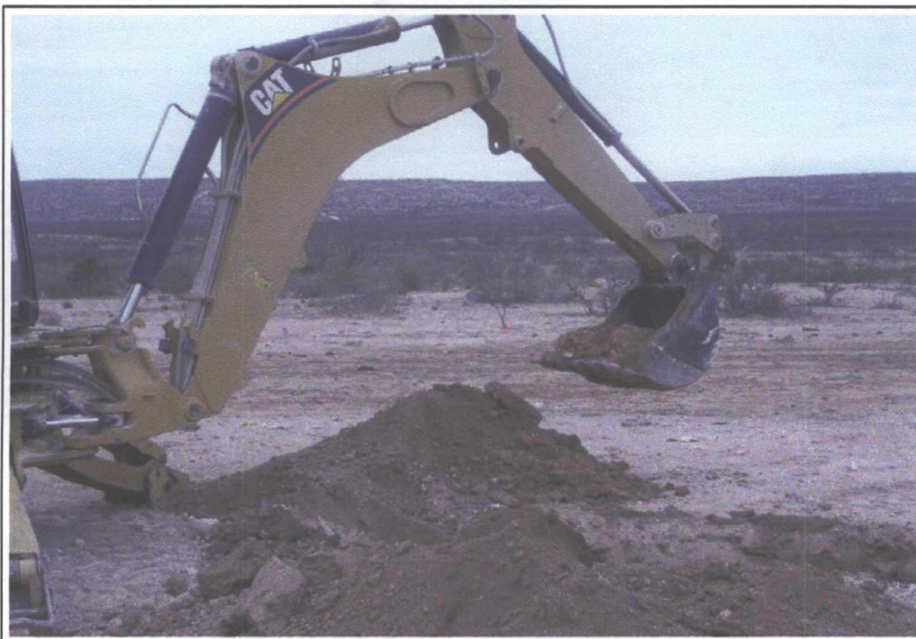
6. Soil samples were collected from the backhoe bucket at specified depth intervals during excavation (view to the west).
