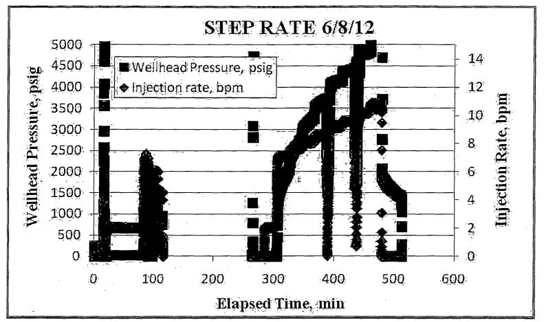
The plot shows the sequence of the step rate test (SRT) performed on June 08, 2012. The test was started with a distributed temperature sensor (DTS) run on a slick line. The test at the injection rate of 2 bpmwas going well, however, as the rate was increased to 7 bpm, the tension in the sensor line caused the bottom hole test measurements to be aborted. The test was performed successfully as planned by measuring surface data only.
