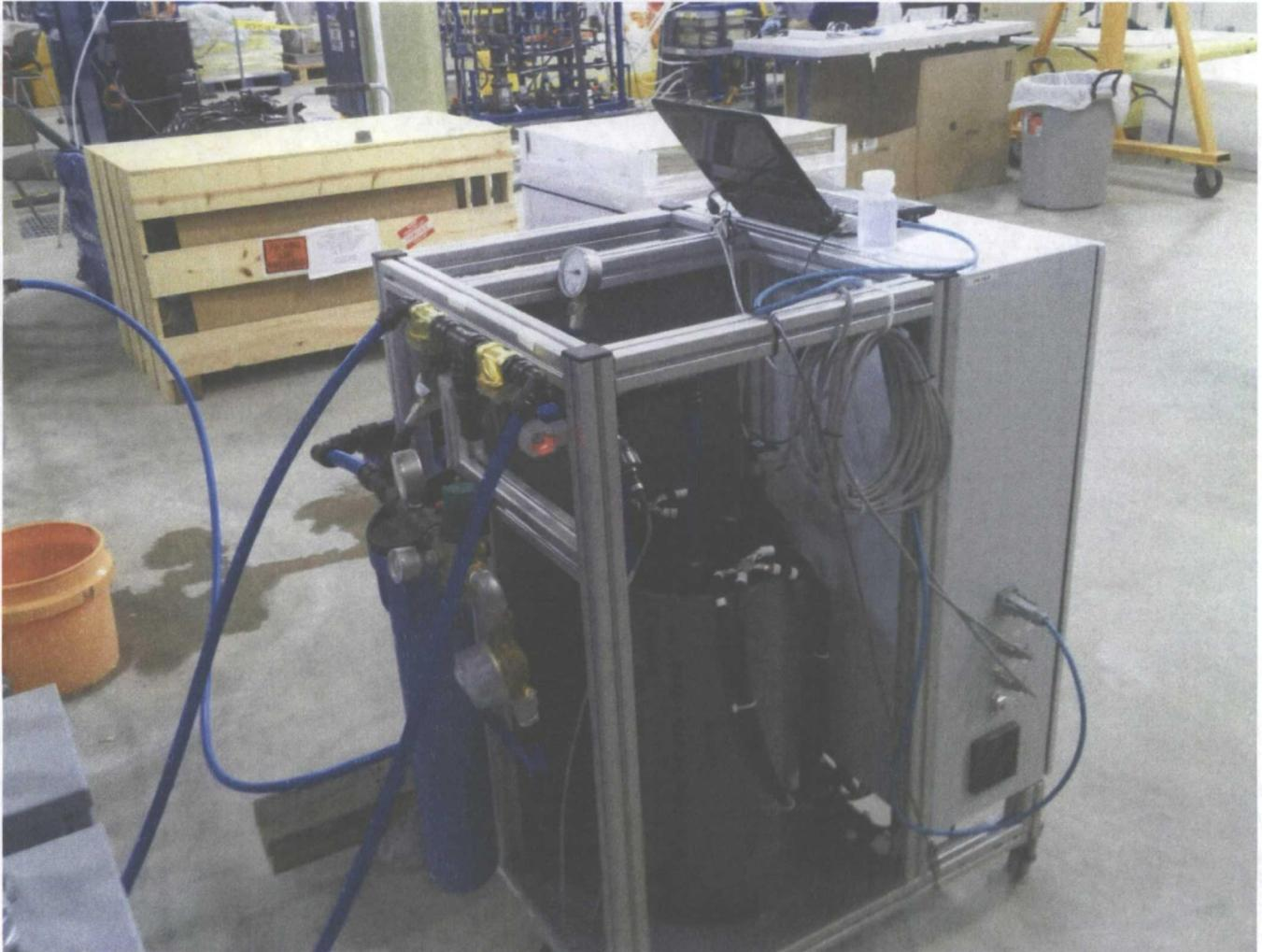
Figure 3. Voltea CapDI system (as installed for brackish water desalination experiments)
