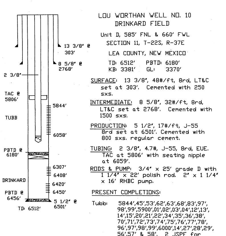
HISTORY: Drilled December, 1949 as a Drinkard gas well. IP'd at top allowable of 98 BOPD and 176 MCFD. Added upper Drinkard pay in 3/74. Acidized 6420-50' and frac'd new perfs 6307'-6408'. IP'd for 1023 MCFD. No record of RBP being removed. Recompleted to Tubb on 8/01/83. Acidized and frac'd perfs 5844 to 6058'. IP'd pumping 30 BD, 28 BLW and 242 MCF per day.
