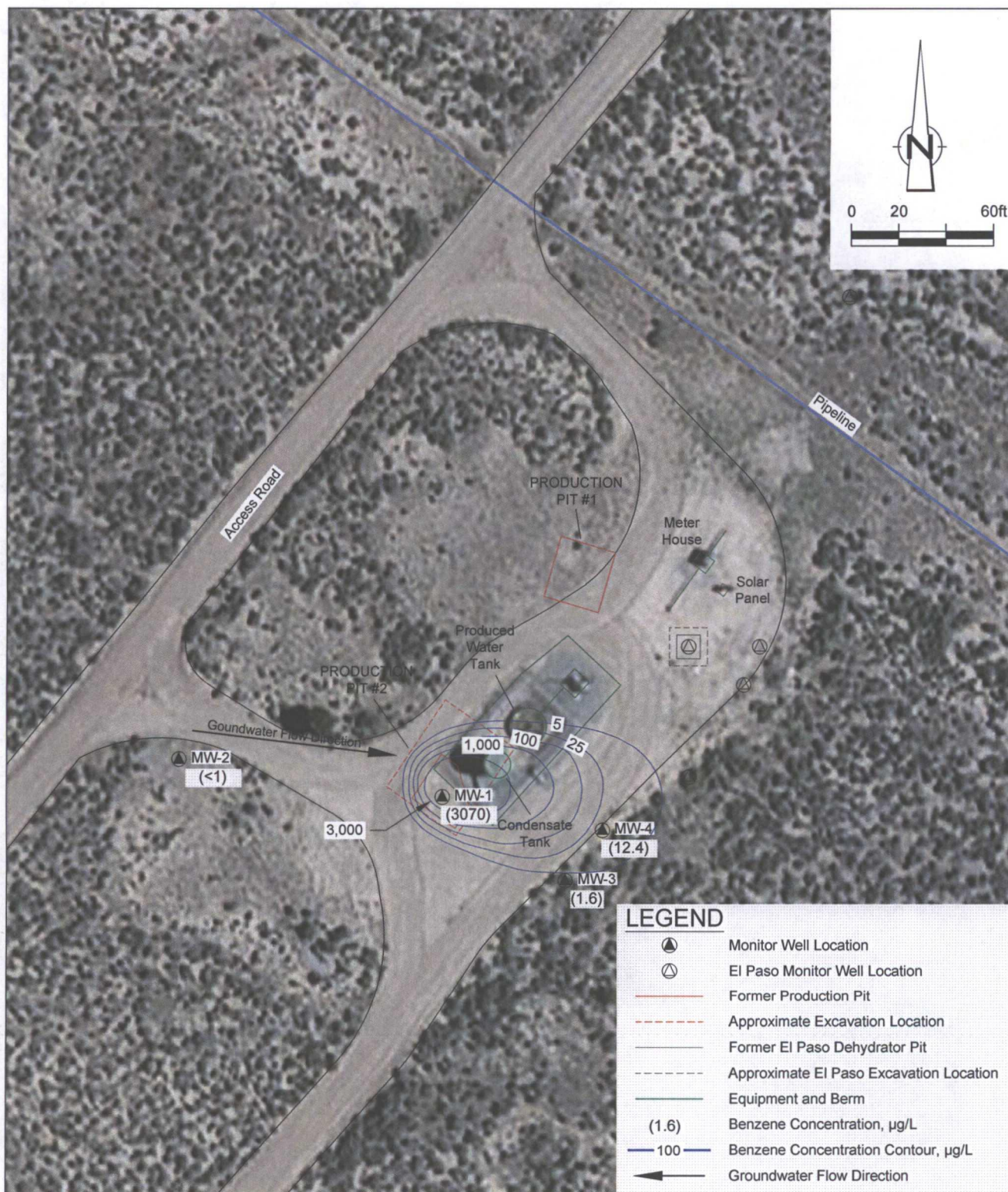
Figure 5 SEPTEMBER 2012 BENZENE CONCENTRATION MAP JOHNSTON FEDERAL No. 4 METERING STATION SECTION 27, T31N-R09W, SAN JUAN COUNTY, NEW MEXICO ConocoPhillips Company
