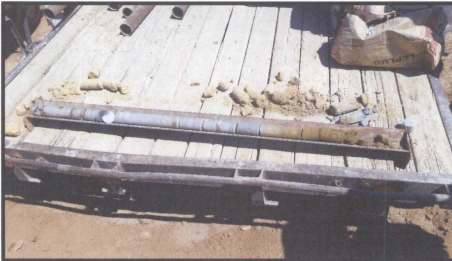
Photo 8: Soil core sample collected from the Trunk K #8 borehole., 43 – 48 feet bgs.
