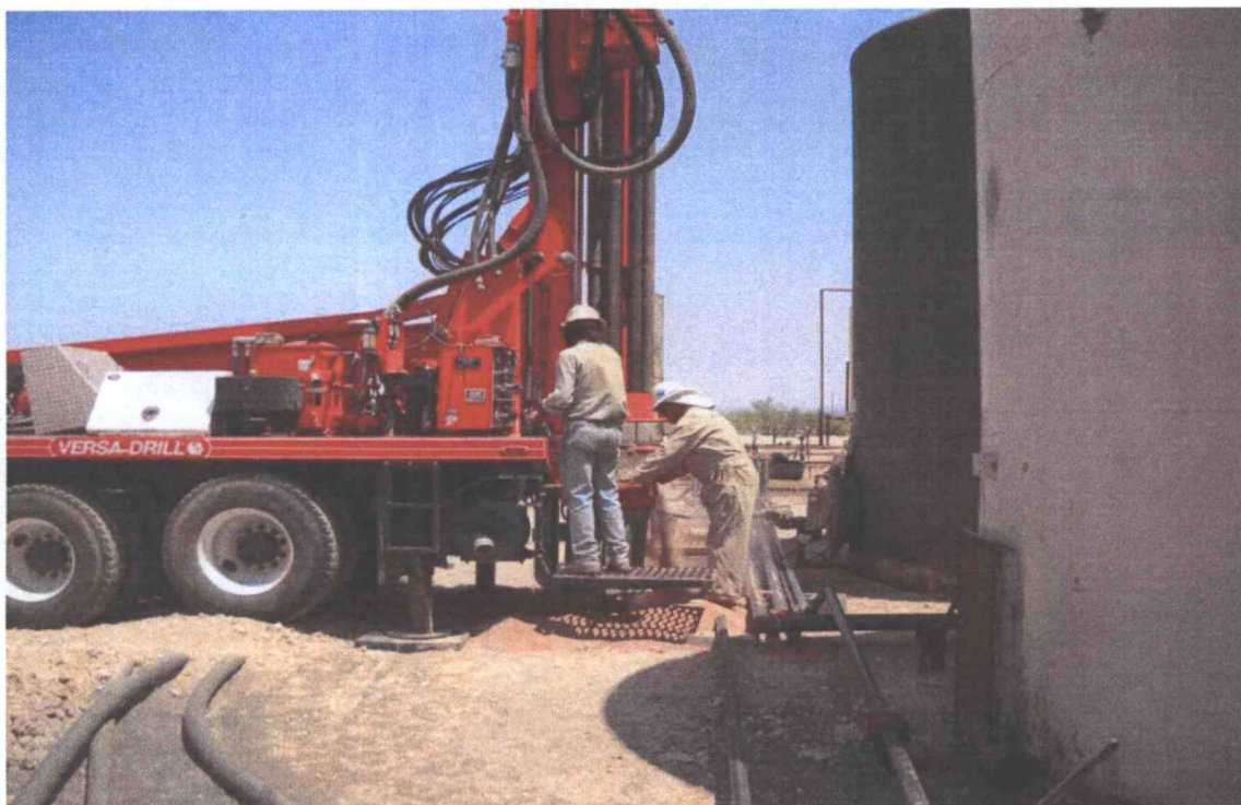
Hat Mesa State 31-32 Battery - Advancement of Soil Boring SB-2
