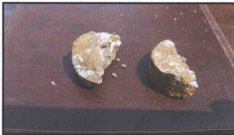
Photo 2: Split spoon sample of the silty clay material containing gypsum and other evaporite crystals.
