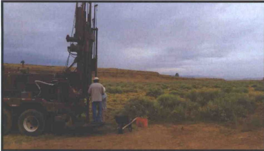
Photo 5: Installing a soil boring near the edge of the disturbed area, in the vicinity of the improperly closed pit.
