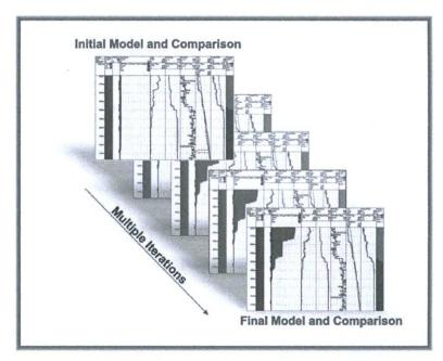
between the theoretical and log data curves indicates that the flow model is in agreement with the log data and the actual well production profile. Discrepancies between the theoretical and raw data curves can be due to tool deficiencies, conflicts between the parameters or conditions that make the underlying empirical models (such as flow regimes) less applicable.
