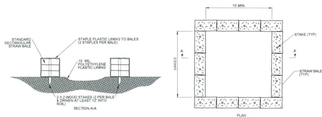
CONCRETE TRUCK WASH OUT FACILITY **CTW**
