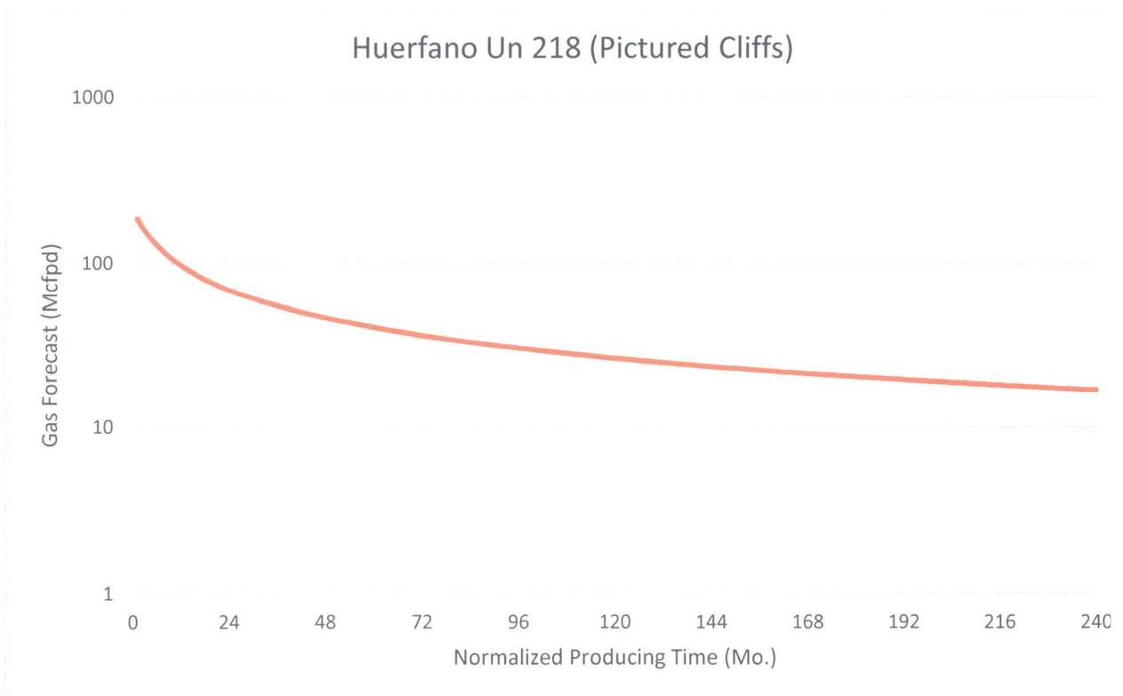
The forecast for Pictured Cliffs production has been generated using a type curve of PC gas production in the surrounding production trend.
