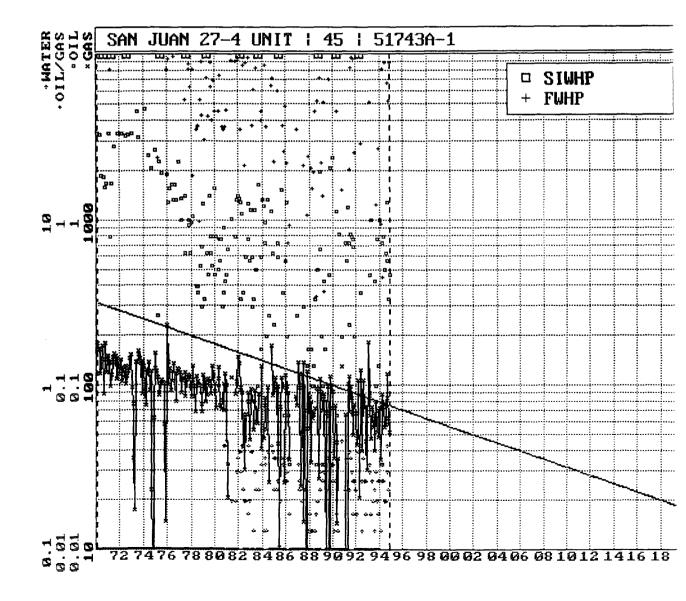
Bottom Hole Pressures Flowing and Static BHP Cullender and Smith Method Version 1.0 3/13/94
