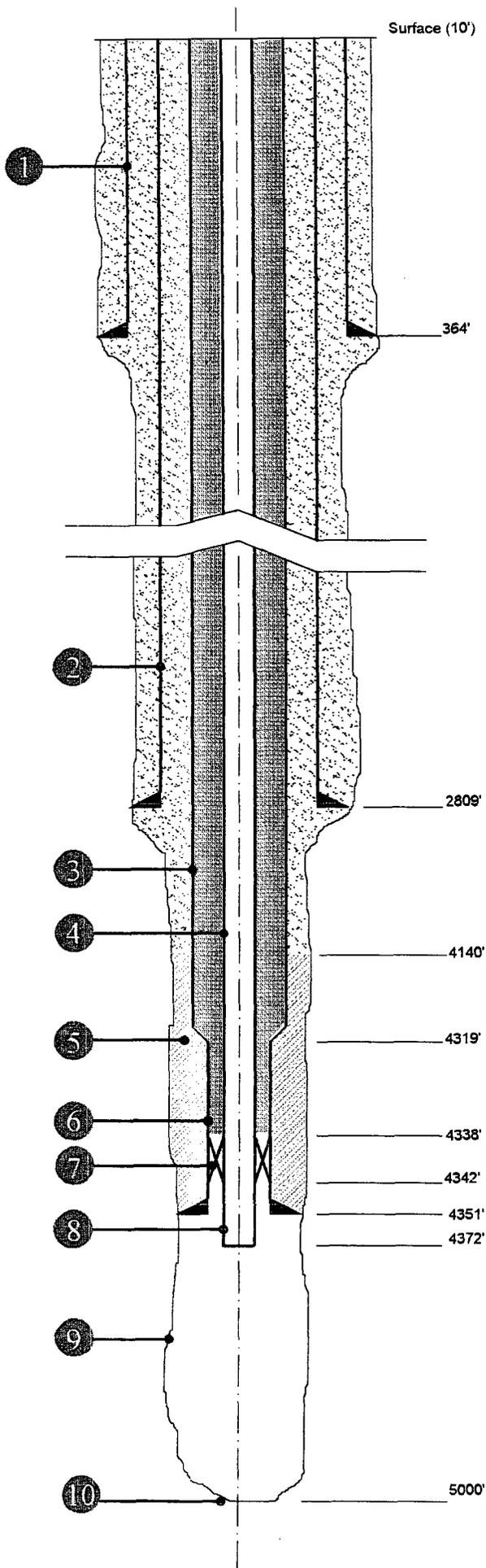
1. Surface Casing: 13-3/8" O.D., 54.5#/ft, J-55, ST & C set to 364' in 17-1/2" hole. Cemented to surface with 350 sacks of Class "C" cement with 2% calcium chloride and 1/4#/sack Flocele.
