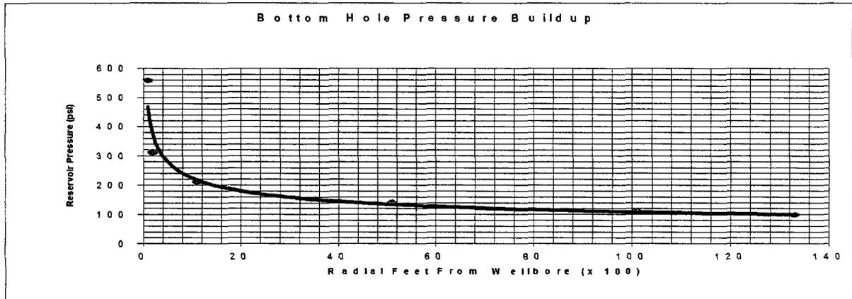
By using the principle of super-imposing pressures, it is possible to estimate the pressure at a point due to the influence of multiple wells. KEDA considered three models in their study:
