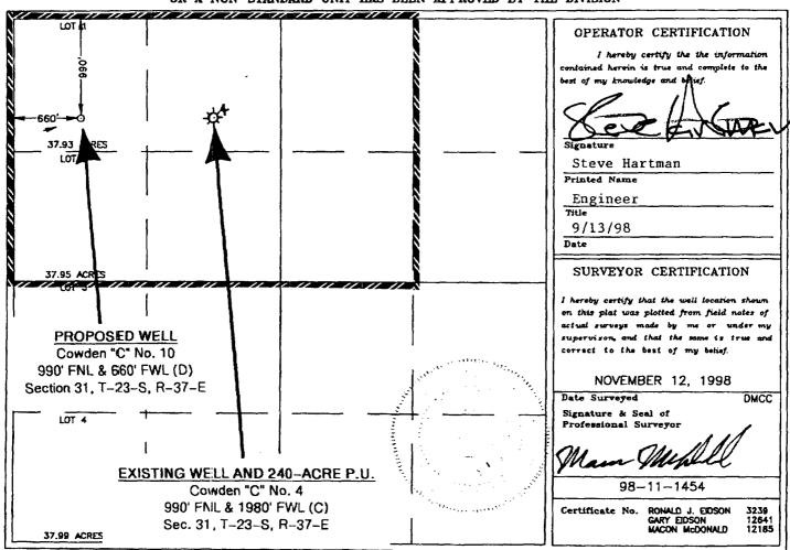
\*Note: Cowden "C" #4 to be squeezed and abandoned upon completion and connection of Cowden "C" #10.
