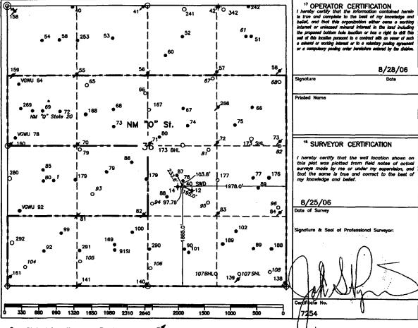
• = Staked Location • = Producing Well = Injection Well • = Water Supply Well -- Plugged & Abandon Well ◎ = Found Section Corner, 2 or 3" iron Pipe & GLO B.C. o = Found /4 Section Corner, 1" Iron Pipe & GLO B.C.
