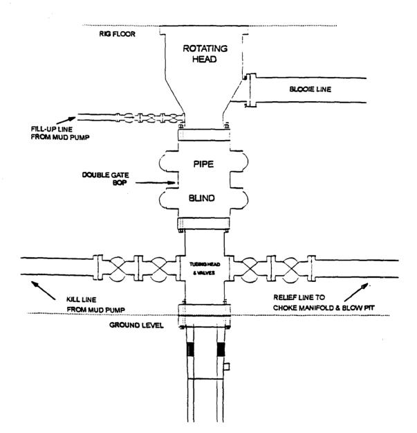
Minimum 8OP installation for Completion operations. 7 1/16" Bore (6" Nominal), 2,000 psi minimum working pressure double gate BOP to be equipped with blind and pipe rams.
