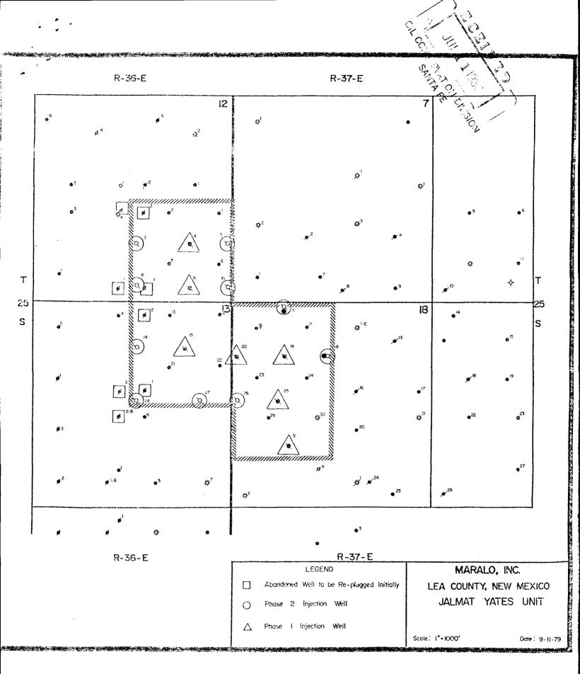
New locations forms C-102 dated June 6, 1980, reflect adjusted location of wells #11 seventy-two (72) feet south and #18 sixty-one (61) feet west of unorthodox locations approved by N.M.O.C.D. Order No. R-5816.
