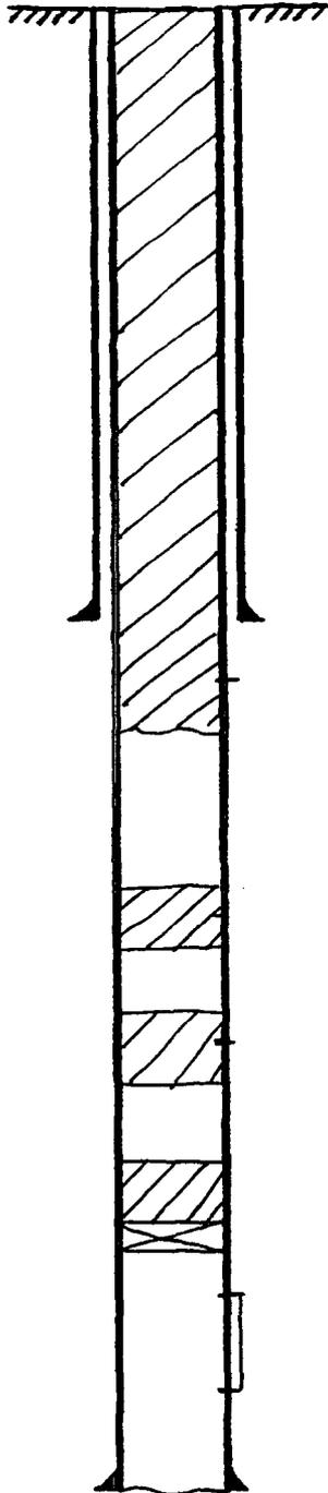
$8\frac{5}{8}$ " casing set at 361' with 175 sx of \_\_\_\_\_ cement
