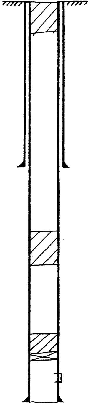
*9 5/8* " casing set at *392* ' with *175* sx of \_\_\_\_\_ cement
