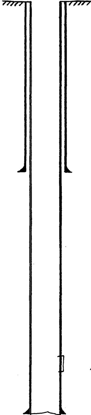
8 5/8 " casing set at 401 ' with 300 sx of \_\_\_\_\_ cement
