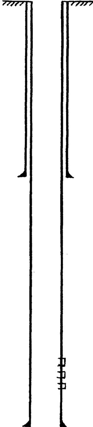
8 5/8 " casing set at 380 ' with 350 sx of \_\_\_\_\_ cement
