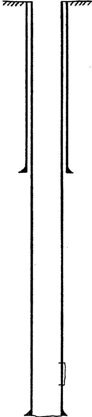
8 5/8 " casing set at 417 ' with 250 sx of \_\_\_\_\_ cement
