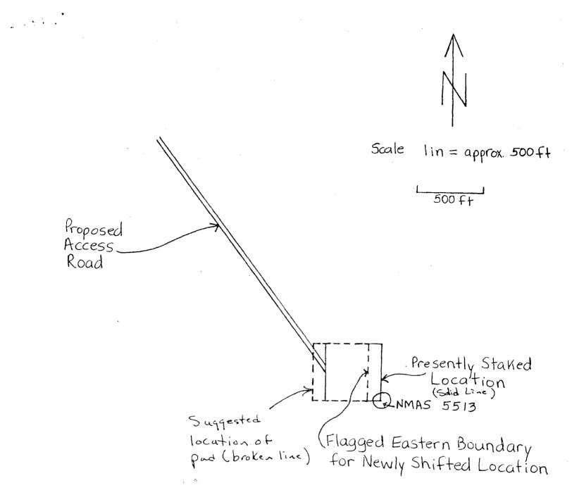
Fig. 1. Schematic representation showing HNG OIL COMPANY's proposed Vcac 13 Federal Well No. 1 vis a vis NMAS 5513 and the proposed location of the pad. NMAS <u>suggests</u> that the location be moved 100 ft to the west from its presently staked position; i.e., 1880 FWL, 660 FNL, Section 13, T25S, R33E.
