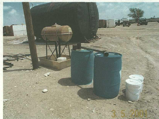
Pic #8- Chemical drums; Brine tank shown in background. Brine tank has liner under tank.
