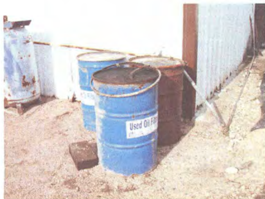
Image 1: Barrels behind truck shop without secondary containment.
