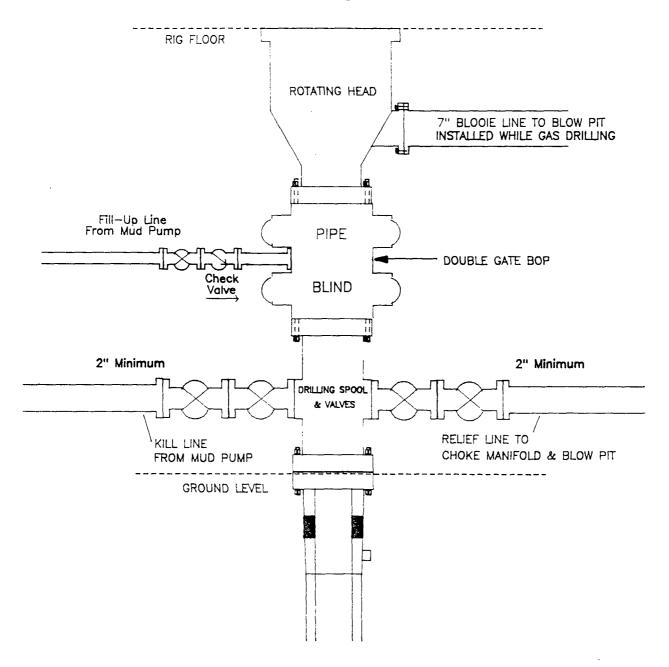
Minimum BOP installation for a Mesaverde well from Surface to Total Depth. 11" Bore, 2000psi minimum working pressure double gate BOP to be equipped with blind and pipe rams. A Schaffer Type 50 or equivalent rotating head to be installed on the top of the BOP. All equipment is 2000psi working pressure or greater.
