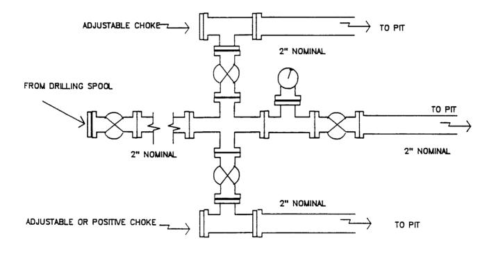
Minimum choke manifold installation for a typical Pictured Cliffs well from surface to Total Depth. 2", 2000psi working pressure equipment with two chokes.
