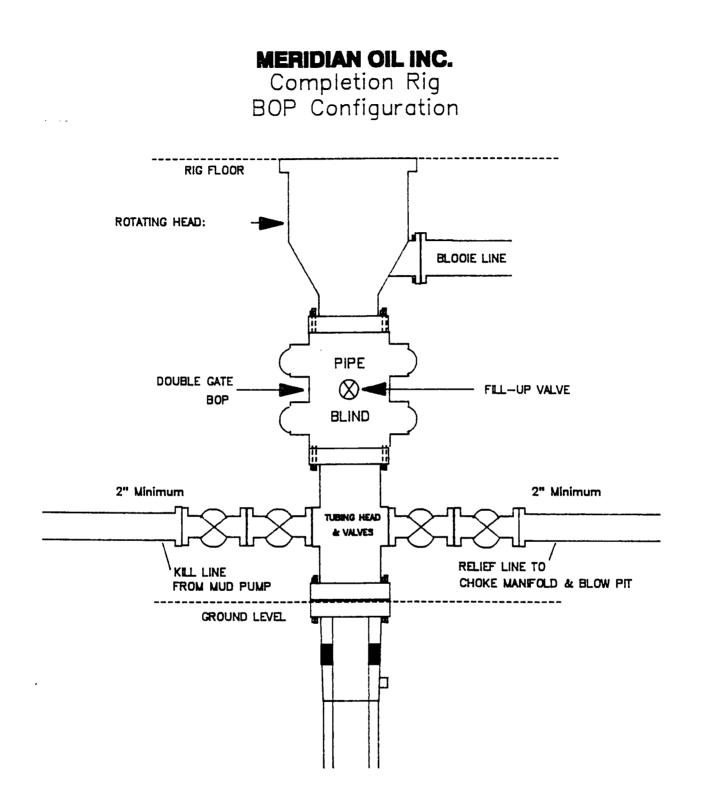
Minimum BOP installation for Completion Operations. 7 1/16" Bore (6" Nominal), 2000psi minimum working pressure double gate BOP to be equipped with blind and pipe rams.
