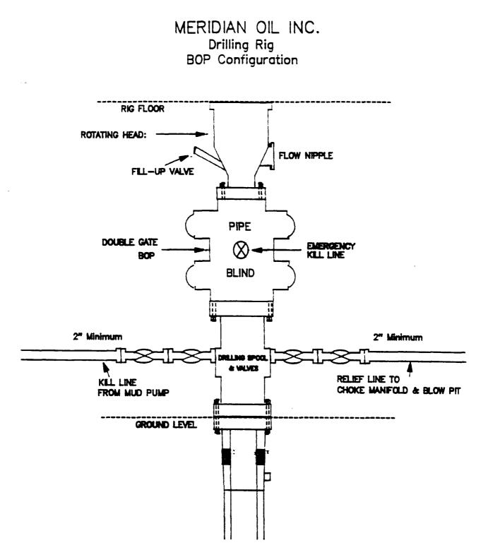
Minimum BOP installation for a typical Pictured Cliffs well from surface to Total Depth. 11" Bore (10" Nominal), 2000psi minimum working pressure double gate BOP to be equipped with blind and pipe rams. A Schaffer Type 50 or equivalent rotating head to be installed on the top of BOP. All equipment is 2000psi working pressure/or greater.
