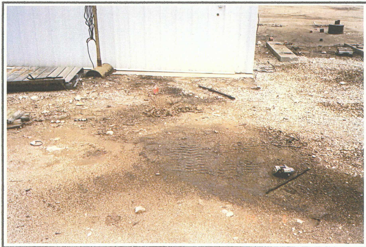
Photograph 10: Additional stained soil was identified to the west of the Machine Shop near the Bucking Machine area (Sample 1-8).
