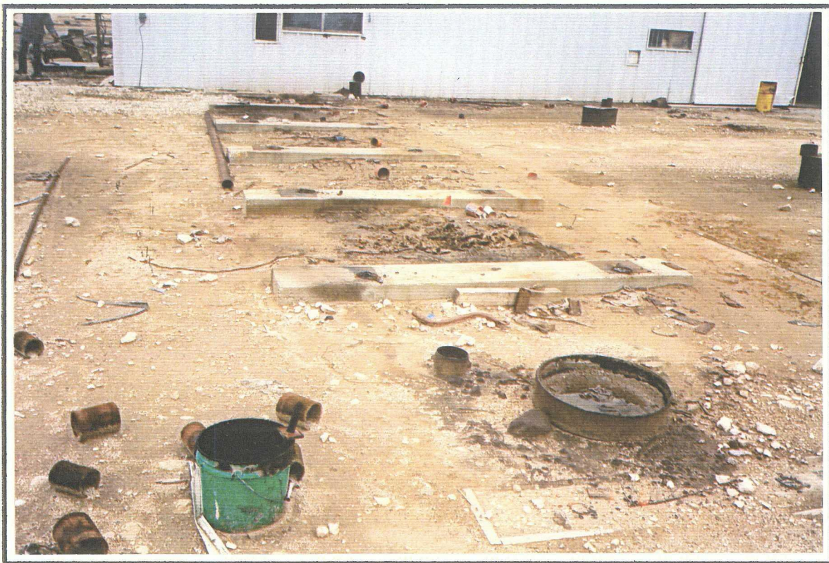
Photograph 9: The ground surface beneath the former Bucking Machine area was hydrocarbon stained (Sample 1-7).
