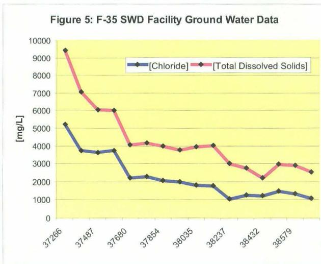
Figure 5: Analytical Results from the F-35 Monitoring Well.
