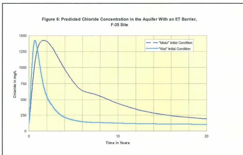
*Figure 6: Predicted Chloride Concentration in the Aquifer With an ET Barrier, F35 Site.*
