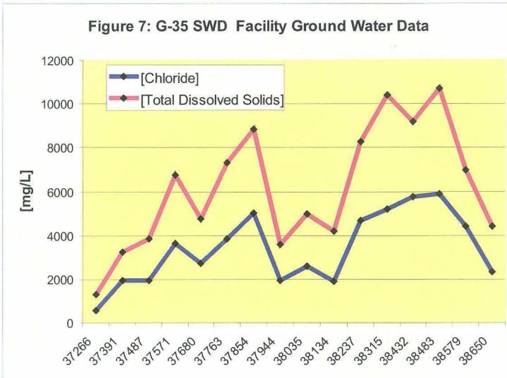
*Figure 7: Analytical Results from the G-35 Monitoring Well.*
