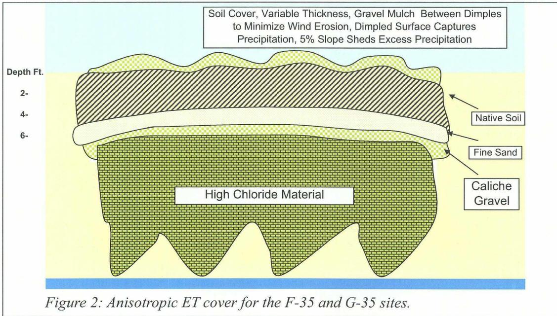
Figure 2: Anisotropic ET cover for the F-35 and G-35 sites.
