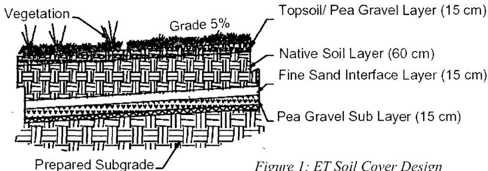
*Figure 1: ET Soil Cover Design from SNL Report SAND 2000-2427.*
