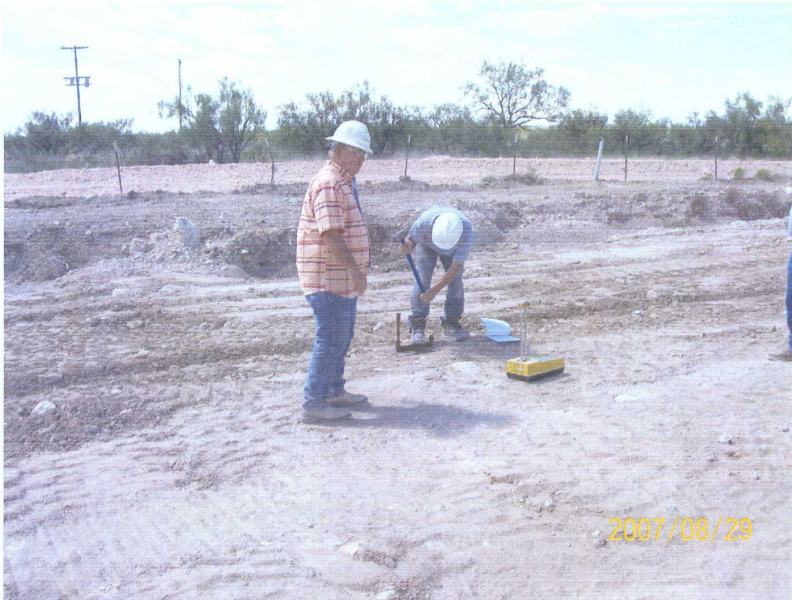
SOUTH EXCAVATION: MEASURING DENSITY OF BLENDED BACKFILL @ 1 ft BELOW GRADE
