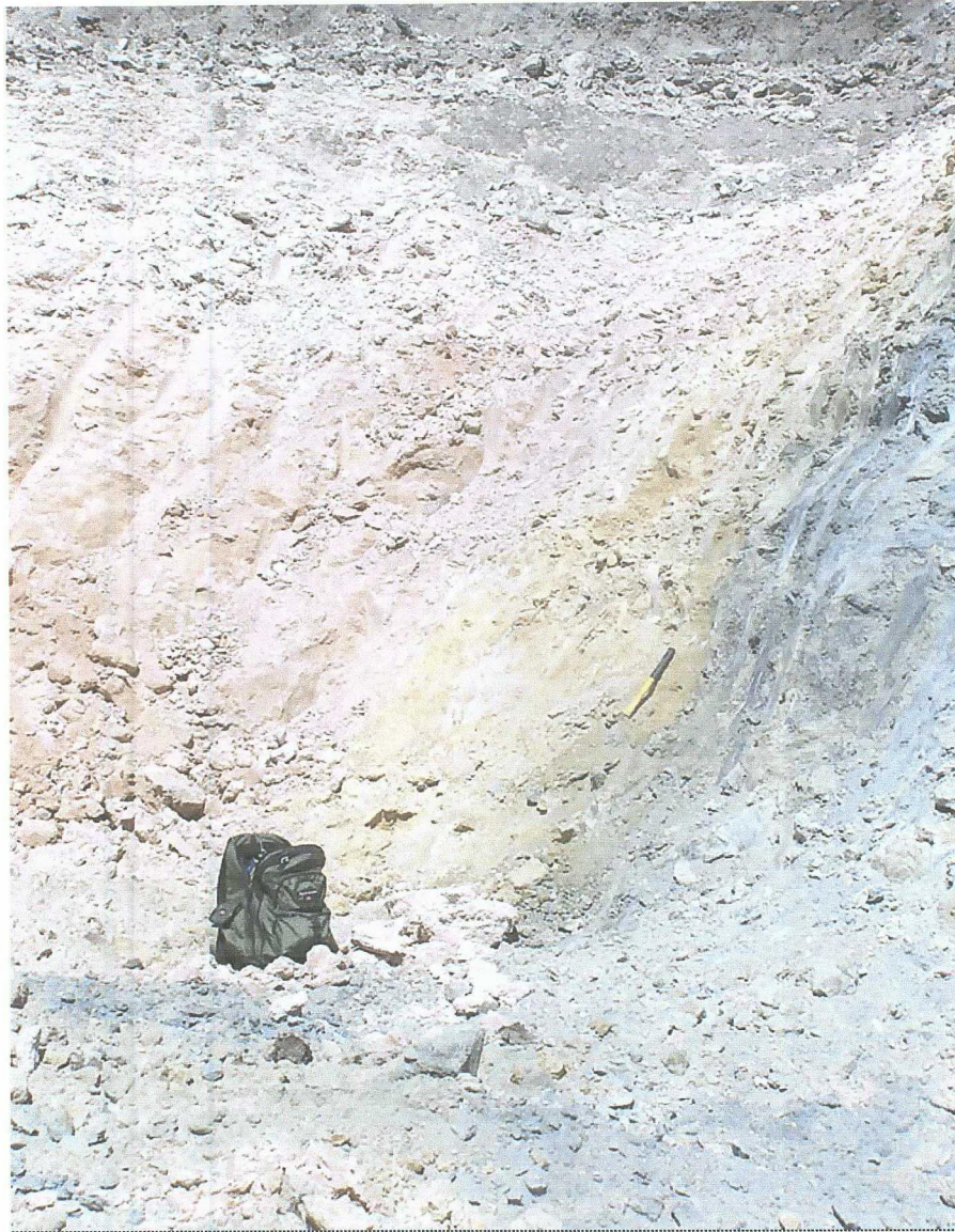
Figure 3. Soil profile inside the excavated pit. The dark area to the right has been darkened due to infiltration of BTEX and brines; the light area at the left has not been affected. The sharp vertical boundary between the dark and light areas is evidence of the limiting soil water content profiles typical for sand soils during three-dimensional infiltration from the tank battery.
