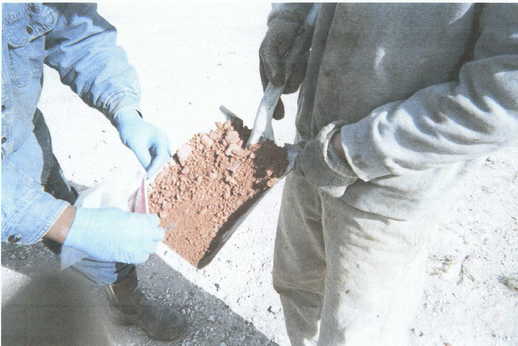
Figure 2 – View of “stiff red clay” substratum, encountered at/near former junction box location.
