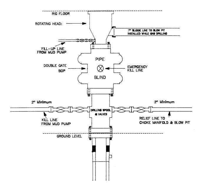
11" Bore, 2000psi minimum working pressure double gate BOP to be equipped with blind and pipe rams. A Schaffer Type 50 or equivalent rotating head to be installed on the top of the BOP. All equipment is 2000psi working pressure/or greater.
