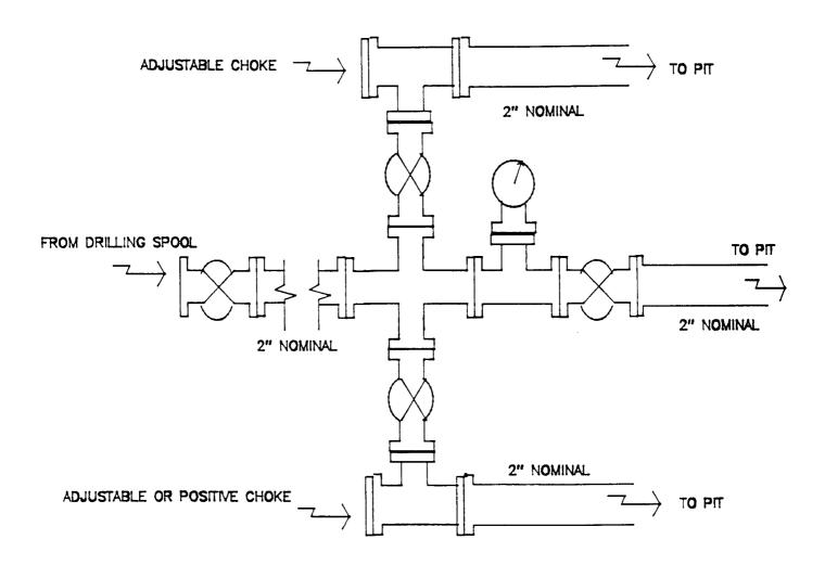
Minimum choke manifold installation from surface to Total Depth. 2" minimum, 2000psi working pressure equipment with two chokes.
