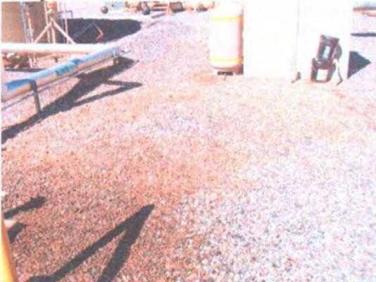
Photo 2: Stained gravel next to submerged sump in Photo 1.
