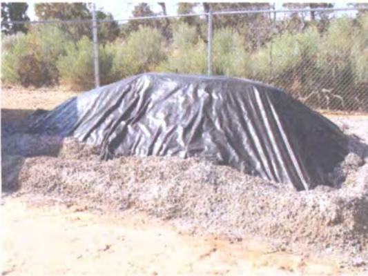
Photo 3: Contaminated soil covered in plastic.
