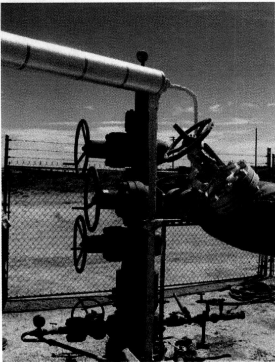
Wellhead w/ blow-out preventers
