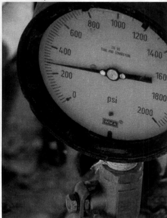
Pressure gauge reading ~300 psig pre-MIT
