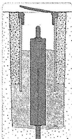
**It's even extendible!** 3' (914mm) lengths of Top Security Sleeves can also be connected together by Berntsen's exclusive End Cap Alignment Bushings and a little PVC Cement. When used in combination(s), nearly any even-foot length over six feet long (1.83m) of support for the rod marker is possible. That's innovative and flexible design at work for you.
