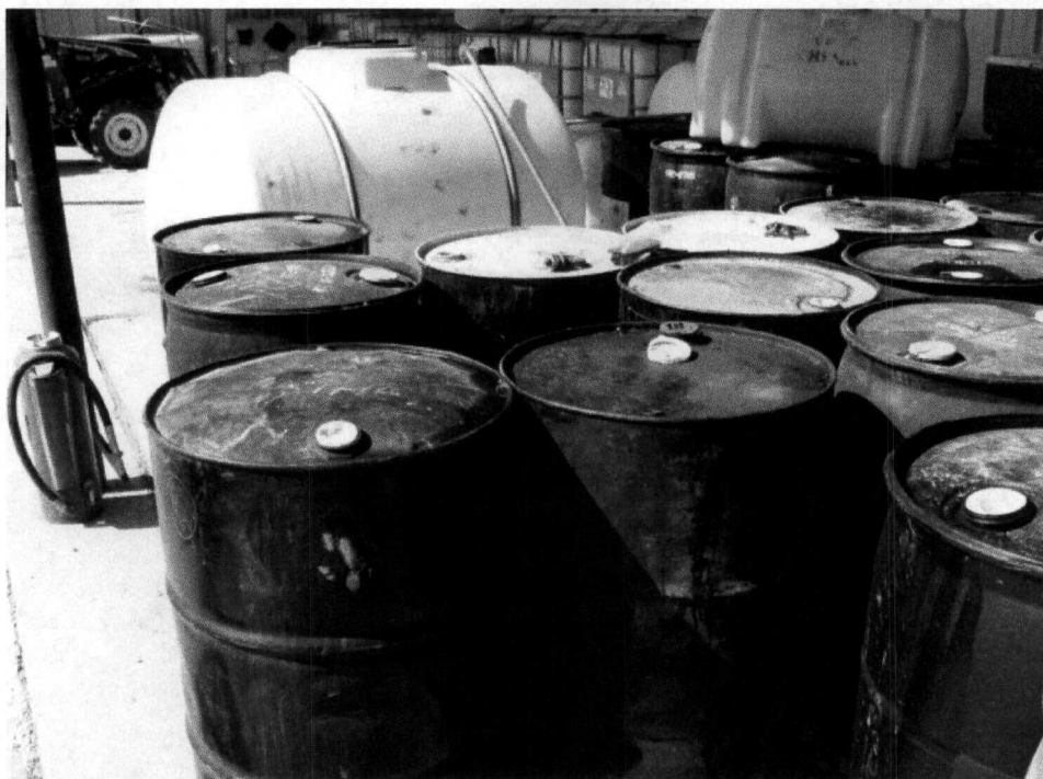
Photo 3: Bulging barrels in storage area.
