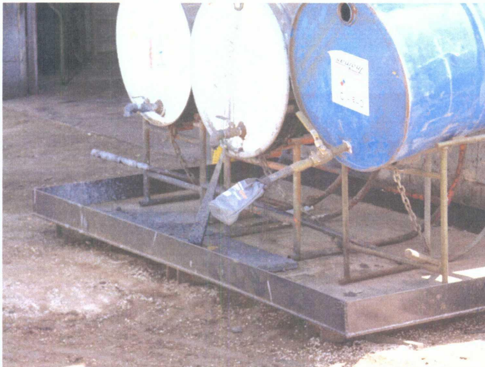
Photo 2 - After; scraped up oil staining, applied absorbent wrap (DuraSorb Small Filter Sock)
