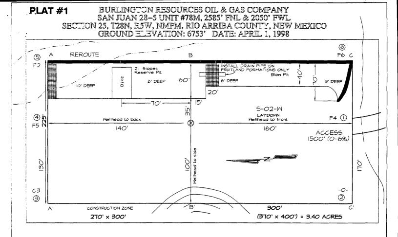
Reserve Pit Dike: to be 8' above Deep side (overflow - 3' wide and 1' above shallow side). Blow Pit: overflow pipe halfway between top and bottom and to extend over plastic liner and into blow pit.
