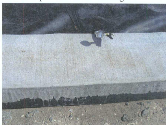
Tank 437 Pressure gauge set into double seam
