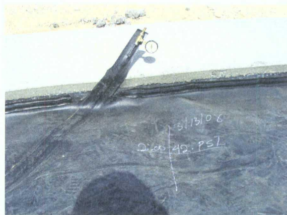
Tank 437 Pressure test in progress between seams w/ test results recorded on liner w/ white chalk
