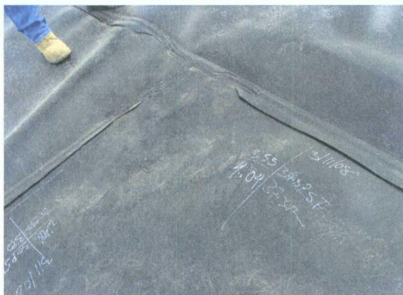
Tank 437 pressure test results in white chalk
