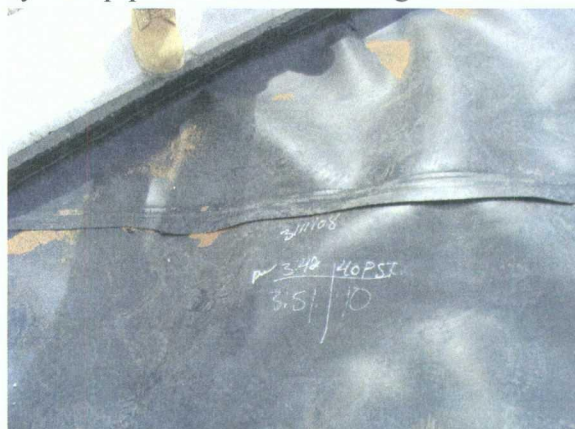
Tank 437 pressure test results near perimeter
