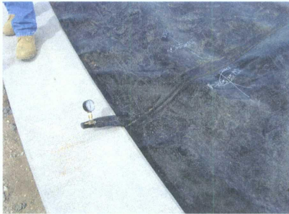
Tank 1225 Concrete ring 1.5 dia. w/ 5 min. pressure test on double welded seam at 30 psi on 60-mil HDPE liner system
