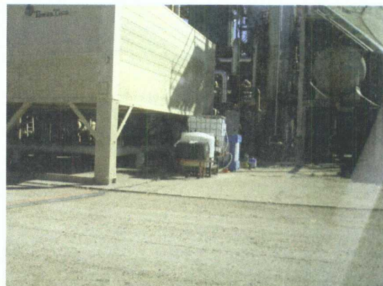
FCC no secondary containment (concrete pad) of totes
