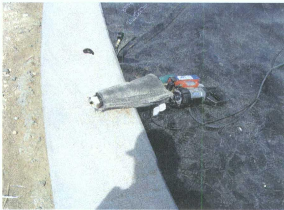
Tank 437 Pressure test in progress w/ pressure gauge between liner seams holding pressure
