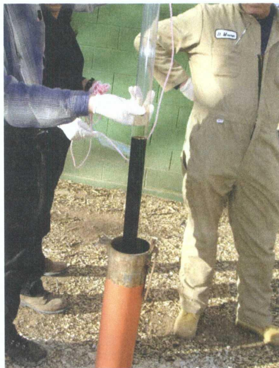
KWB-8 Gas odor touch bottom of well, pure product in well
