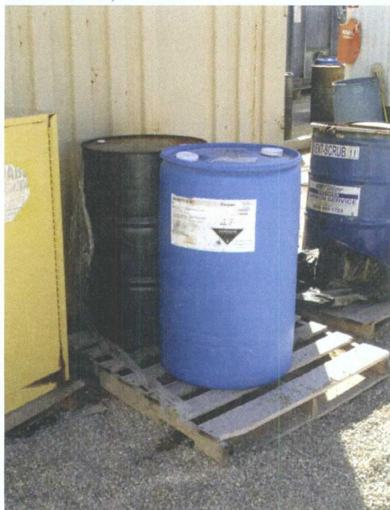
Improper storage of totes (no secondary containment) WWTP
