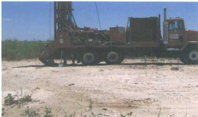
View facing southeast showing drilling of soil boring B-4.
