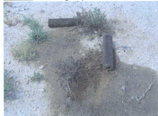
Photo 5: Used filters and soil staining.
