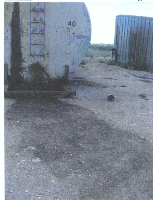
Photo 6: Staining from frac tank valve.
