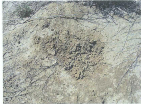
Photo 16: Dry drill cuttings located on ground.
