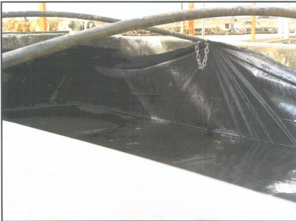
Mud tank (roll-off bin) with floating oil, April 2009
