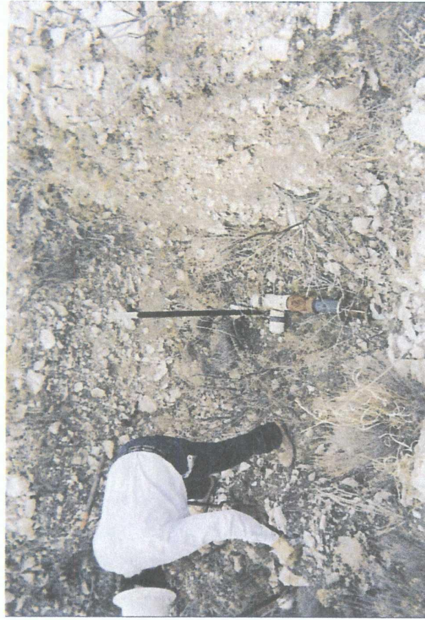
taking a 4-wall composite sample
